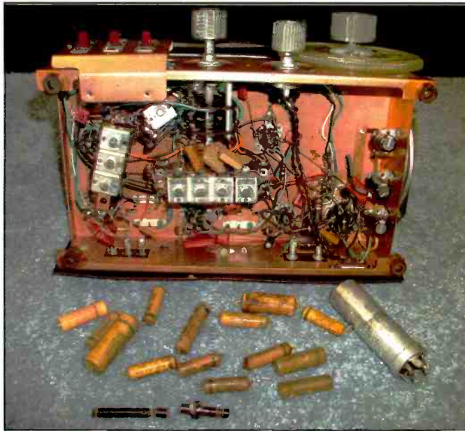
Photo F. All of the old paper and electrolytic capacitors were replaced.
