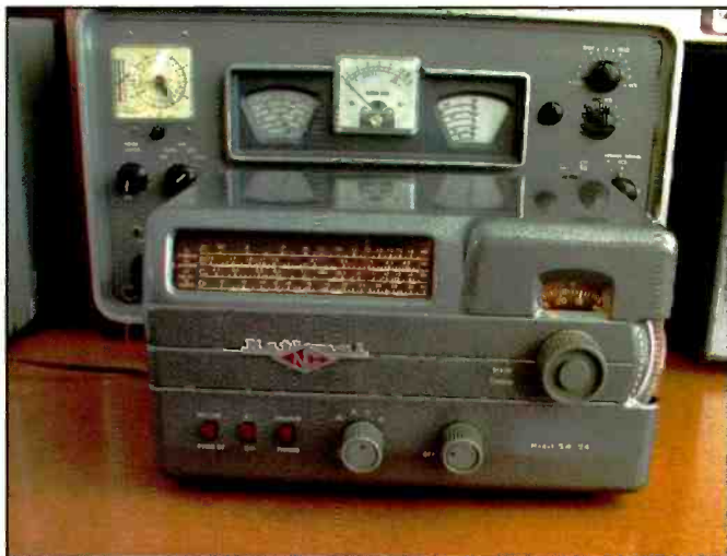
Photo H. The restored National SW-54 is a cute little set. The Lucite dials are brightly illuminated with a single #47 lamp.
