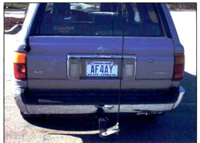
This photo shows the rear NMO-27 antenna that I use for 10 meters. The mount is a Diamond brand. The receiver hitch I made from several parts and I can interchange "Hamstick" HF antennas for whatever band I choose. Both of these antennas go to the Yaesu FT-900 and I use an MFJ selector switch to select my antenna. My call sign, AF4AY, is also my license plate registration. And, of course, I display several WCU and UNCA Alumni stickers on the vehicle.
