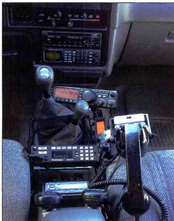
This is the overall view of the radio equipment in the daytime. Note the flush mounting (in the dash) of the PRO-2067 scanner. The three transceivers have the control heads remote mounted and the XM is remote mount as well. I had to use a piece of soft metal strap (similar to plumber's strap) mounting of the spectra microphone.
