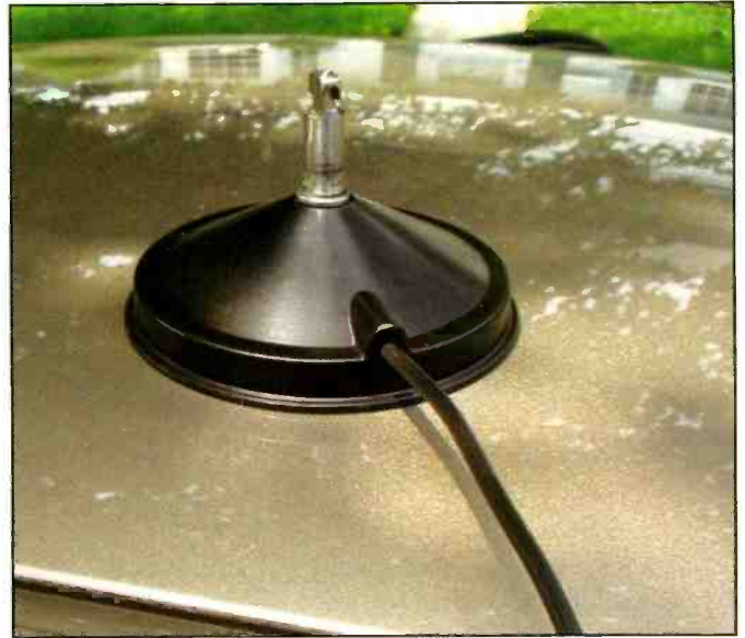
The short stainless steel Quick Disconnect is perfect when garaging your vehicle or stopping in public areas; just push down and twist the assembly, and the antenna comes off for storage.
