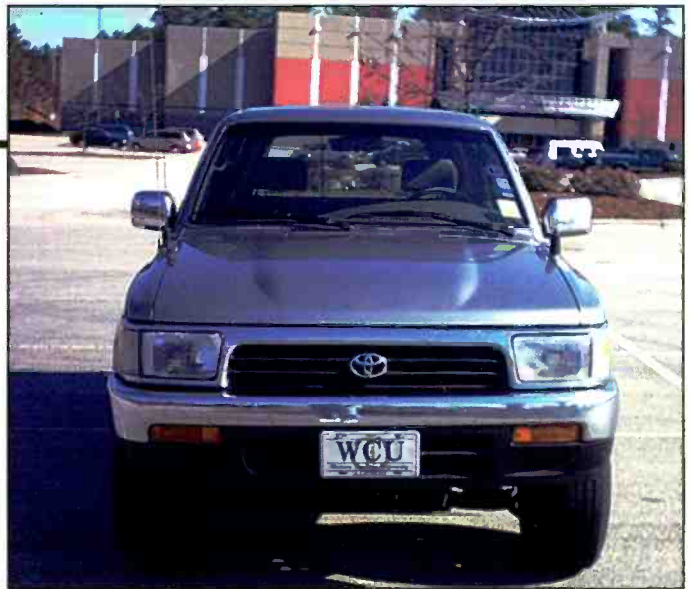
Here's the Larsen NMO 2/70 for the Yaesu FT-7100M and a Larsen NMO-40 that I have for the scanner (I usually monitor NCSHP which is on 42 MHz lowband). I have several antennas that can be interchanged if I am concentrating on 800-MHz trunking. And, finally, my front license plate shows WCU (Western Carolina University Alumni; Master of Public Affairs, class of 2002).
