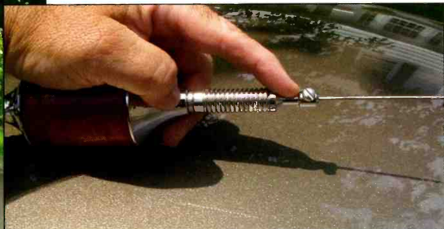
The top stainless steel whip is adjusted with a standard screwdriver; you don't have to hunt for yet another Allen wrench!
