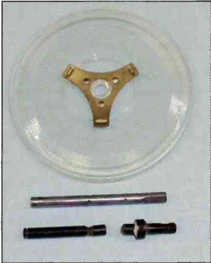
Photo B. The original tuning shaft (bottom) was broken. The collar on the old shaft was broken off the center of the bandspread dial (top). The metal replacement tuning shaft is in the center.
