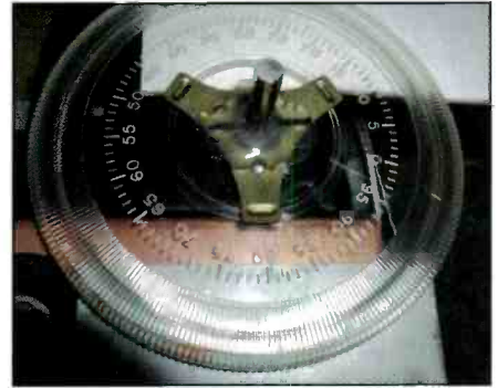
Photo C. The bandspread dial was attached to the new tuning shaft using hot-melt glue.
